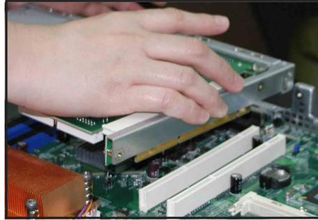
5. If you wish to install a second PCI card, repeat steps 1 and 2 then install the card to the **right bracket** as shown. Secure the card with a screw.
