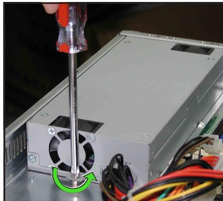
3. From the rear panel, remove the two screws that secure the rear end of the power supply.
