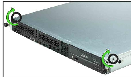
2. Loosen the two thumbscrews on the rear panel to release the top cover from the chassis.
