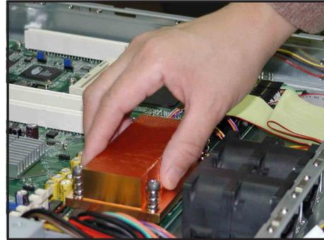
2. Hold down the heatsink lightly and twist each of the four screws with a Philips (cross) screwdriver just enough to attach the heatsink to the motherboard.
