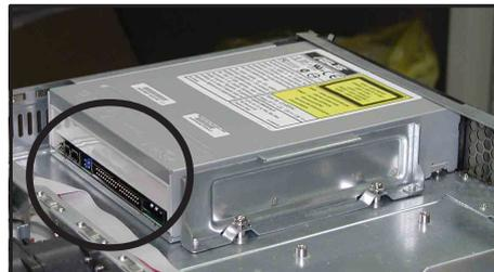
4. Use a Philips (cross) screwdriver to remove the two screws that secure the metal bracket on the side of the ODD.
