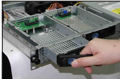
3. Take note of the drive tray holes. Each side has three holes to fit different types of hard disk drives. Use two screws on each side to secure the hard disk drive.
