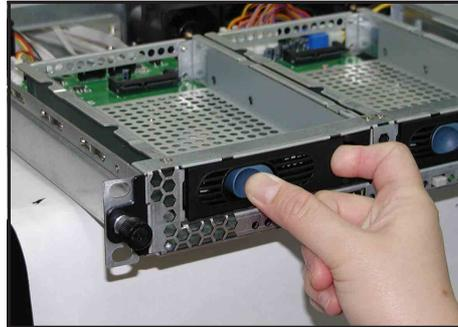
2. Firmly hold the tray lever and pull the drive tray out of the bay.
