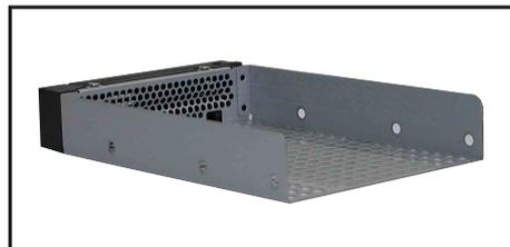
4. Place a SATA hard disk drive on the tray, then secure it with four screws.
