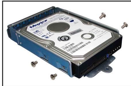
3. Carefully place the tray with installed hard disk drive into the drive bay. Slide it forward until the front end aligns with the front panel, and the screw hole matches the standoff.
