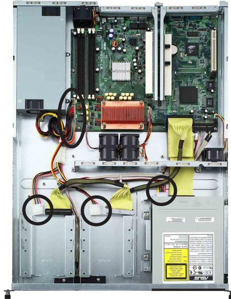
2. Use a Phillips (cross) screwdriver to remove the screw that secures the front end of the power supply.
